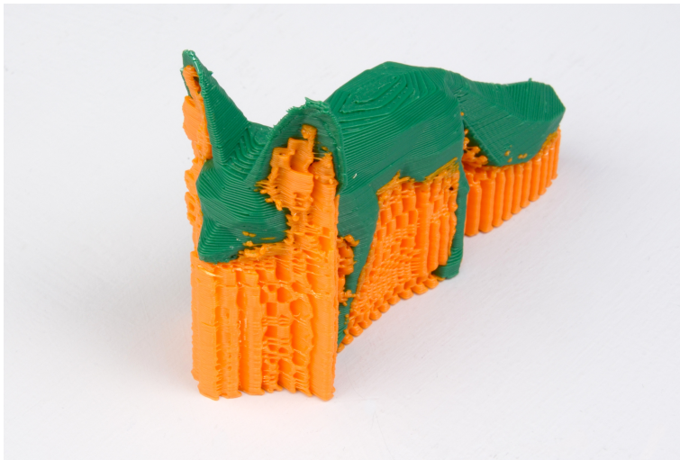
Figure 3.17: An example of an object printed with support material.
