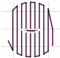
Figure 3.39: Support infill pattern: Rectilinear
