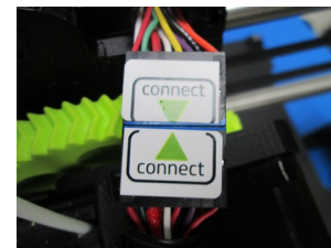
Align the extruder connector and the extruder harness connector
