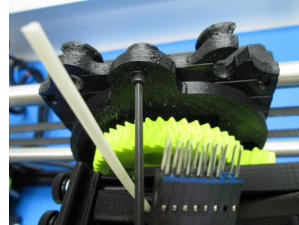
Attach Extruder to the X carriage mount
