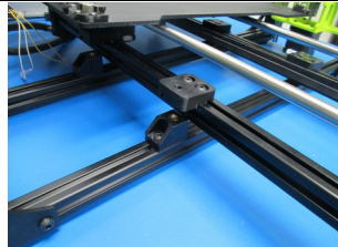
Place the Y assembly on the Z frame assembly.
