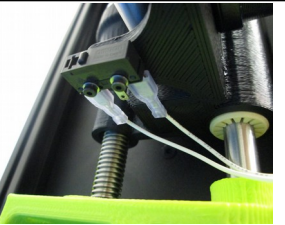
Connect the X Min switch to the X right assembly lower switch
