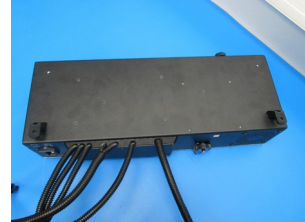
Install two control box mount at the rear of the control box
