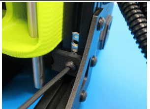
Slide the mounts inside the frame, secure to the extrusion lower T-Nut, tighten control box mount also
