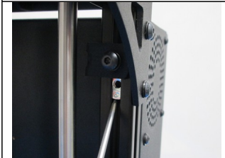
Secure upper T-Nut to the extrusion to hand tight
