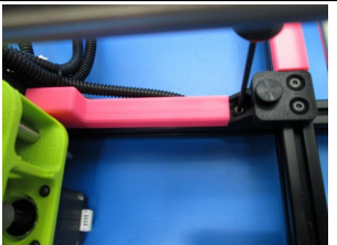
Tighten the screw in each chassis mount.
