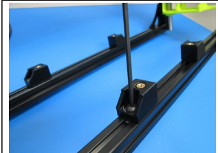
Install Y chassis mounts (2) each on front and back lower extrusions
