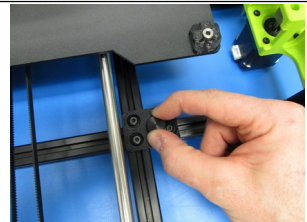
Secure the table mounts to the chassis mounts with thumb screws
