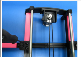
Tighten the two screws in each bed mount.
