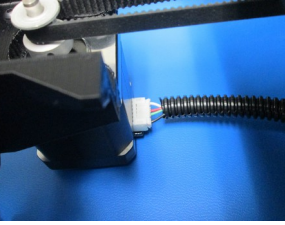
Connect the Y axis cable to the X right motor
