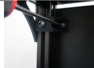
Attach the control box mounts on the front frame to the control box, tighten to hand tight
