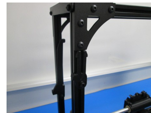
install the feed tube holder as shown
