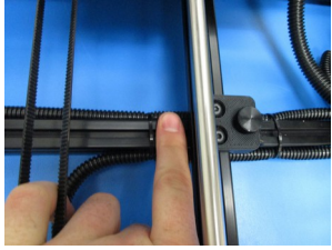
Secure the Extruder harness frame back top extrusion
