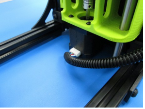
Connect the X left side cable to the X left motor
