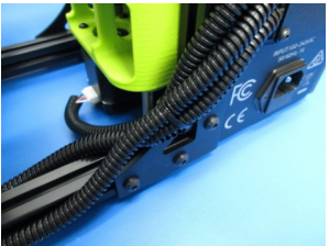
Secure the Z right and Y axis motor harnesses again to the frame cross member just inside the Y axis assembly
