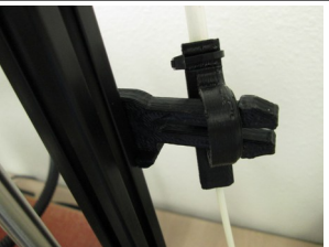
Install the spinner onto the feed tube holder
