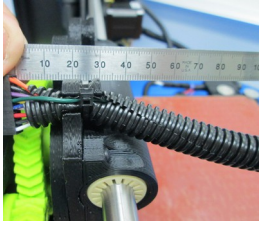
Secure extruder cable onto the extruder mount
