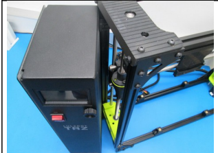
Stand the control box up next to the frame, position mounts to the frame
