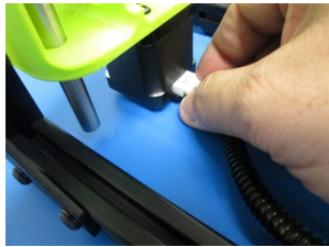
Connect the X right side cable to the X right motor
