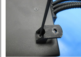
M5x10 BHCS used to attach control box mounts
