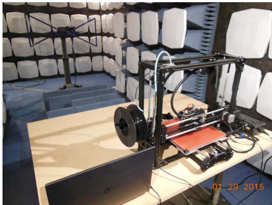
Radiated emissions test setup
